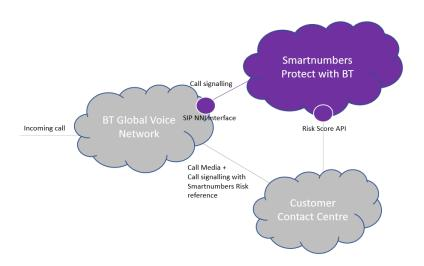
**3.1.2 Plugin Option:** BT will provide and manage the Service for the the risk score calculation and presenting its results via SIP or API as detailed in purple on the below diagram.
