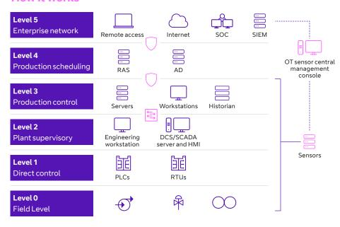
Sensors collect all the data from your OT network and feed it into the management console, alerting you to anomalies and threats. This can also be linked to your SIEM and SOC if required.
