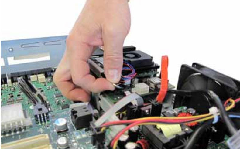
Figure 68: Removing the Battery
