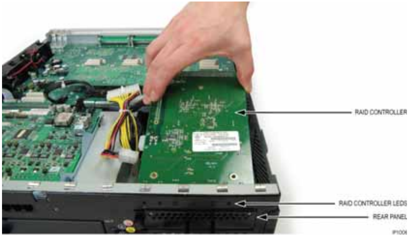
Figure 79: Position the RAID Controller Board
