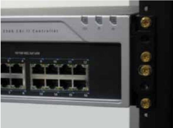
Figure 20: CX II/CXi II Controller Rack-Mount Installation - Fastening Angle Brackets to Rack Frame
