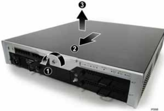
Figure 12: MXe/MXe Server - Removing the Cover
