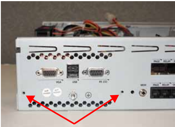
Figure 64: Retaining Hole Locations
