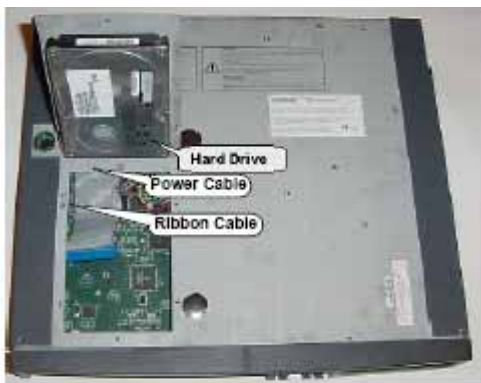
Figure 74: LX Controller Hard Drive Installation
