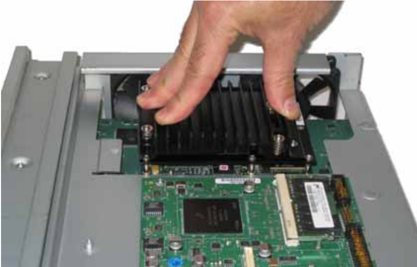
Figure 53: Installing an APC-MXe in the MXe Server
