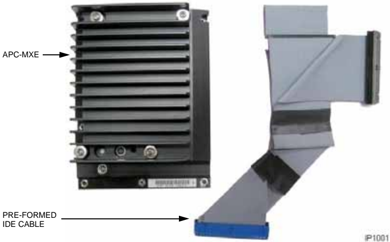
Figure 31: APC-MXe and Pre-formed IDE Cable
