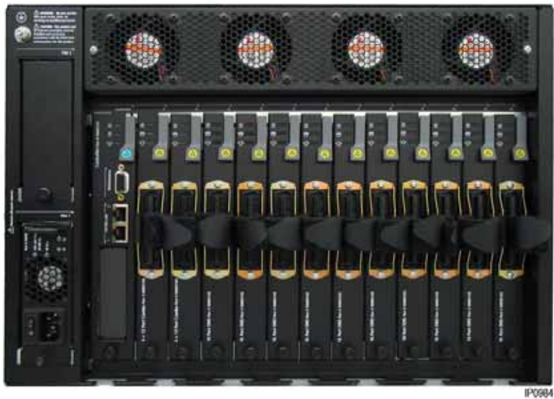
Figure 91: AX Controller – Rear Panel
