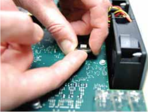
Figure 54: Removing the Battery
