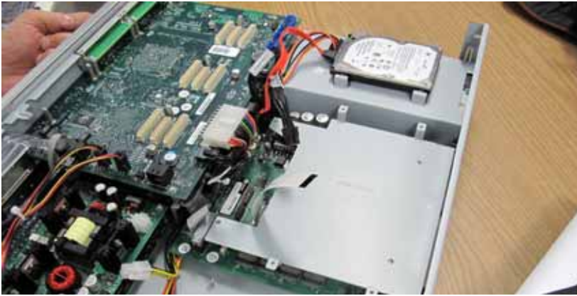
Figure 49: AOB Mounting Plate in Position
