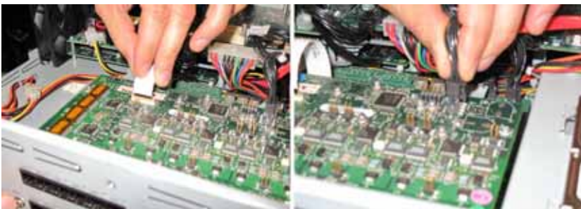
Figure 50: Attach Flex cable and Power Cable to AOB
