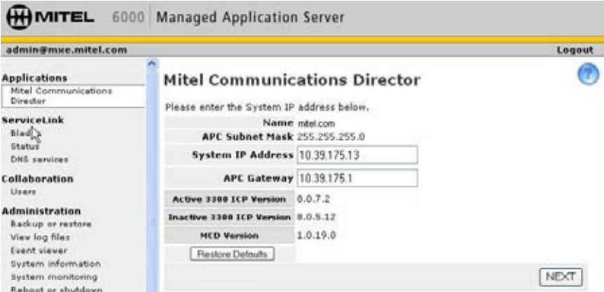
Figure 25: Change the System IP and APC Gateway Addresses
