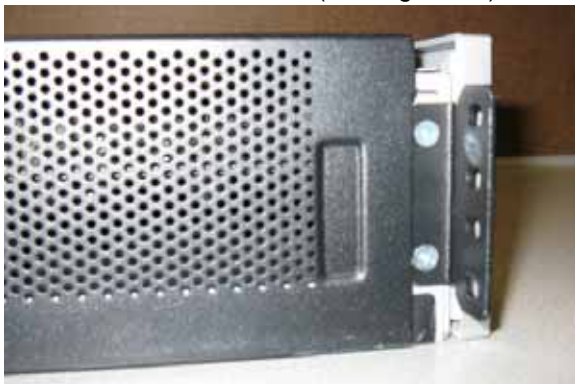
Figure 19: Figure 21: CX II/CXi II Controller Rack-Mount Installation - Attaching Brackets to Controller
