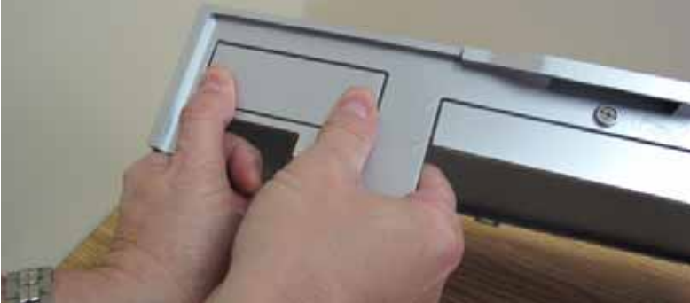
Figure 66: Remove Blanking Plate
