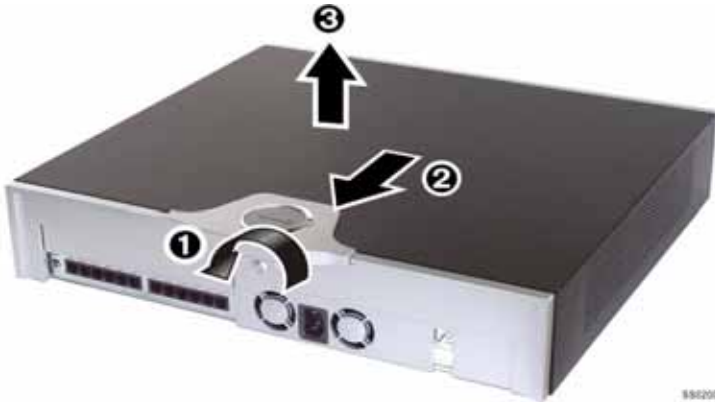
Figure 11: CX/CXi, CX II/CXi II - Removing the cover
