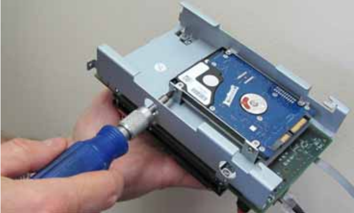
Figure 67: APC-CX(i) II Hard Disk Drive Removal
