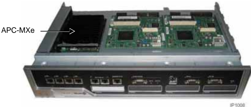
Figure 51: APC-MXe on MXe Carrier Board
