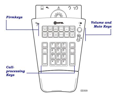
Volume and Mute Keys - used to increase (+) or decrease (-) the ringer volume and the volume of the earpiece in the handset or headset. The Mute key turns the microphone in the headset or handset on or off.
