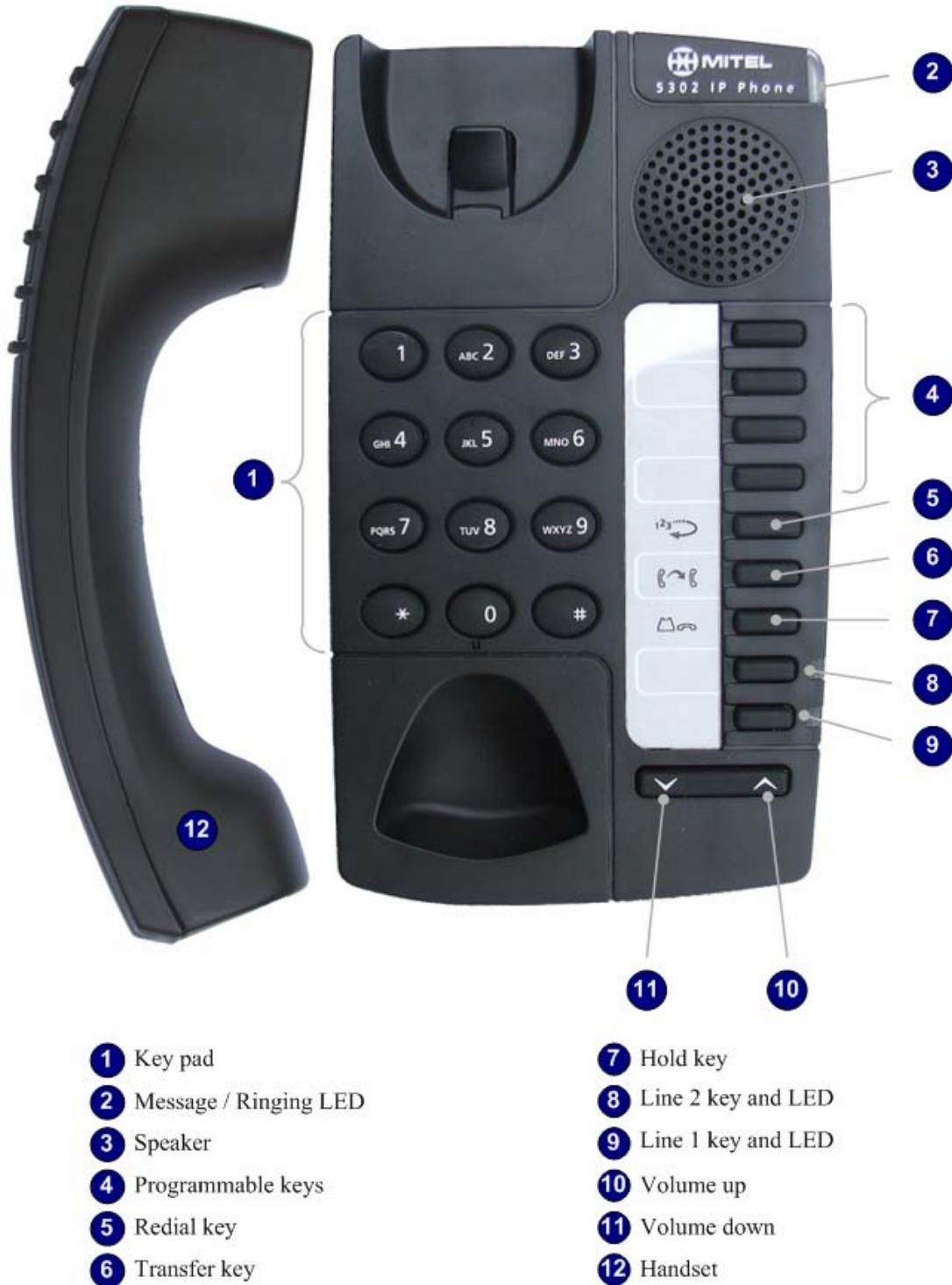
Figure 1: Physical layout of the Mitel 5302 IP Phone
