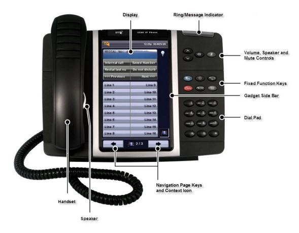
The BT 5360 Systemphone has a seven-inch (17.8 cm), backlit, high-resolution (800 x 480), colour, touch-screen display with brightness controls, on-hook dialling, a hearing aid compatible handset (HAC), and a Ring/Message indicator.
