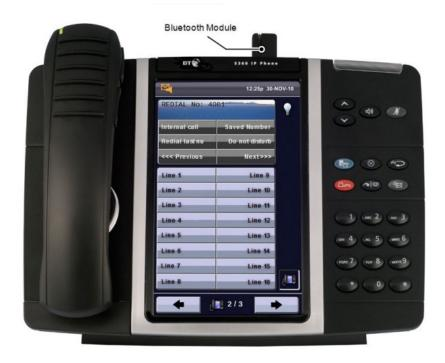
The Cordless Devices Application provides access to the configuration settings and information screens that apply to the Bluetooth module and accessories.
